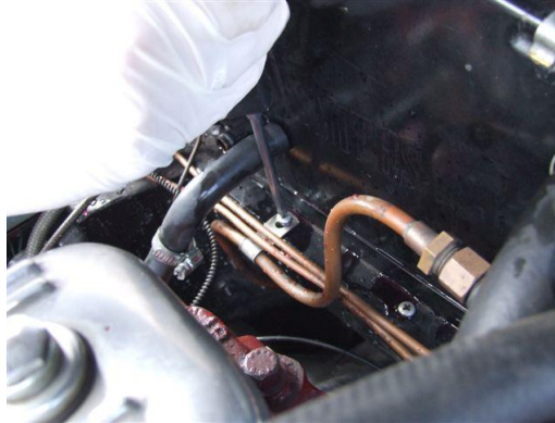
Removing the retaining Screws
