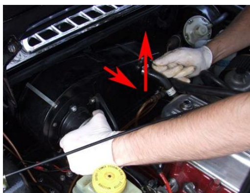
Lifting the heater box
